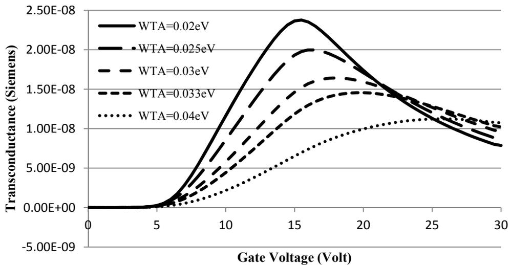
Figure 4: Variation of transconductance as a function of gate voltage for different values of tail states
