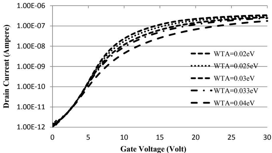
Figure 5: Variation of drain current as a function of gate voltage for different values of tail states
