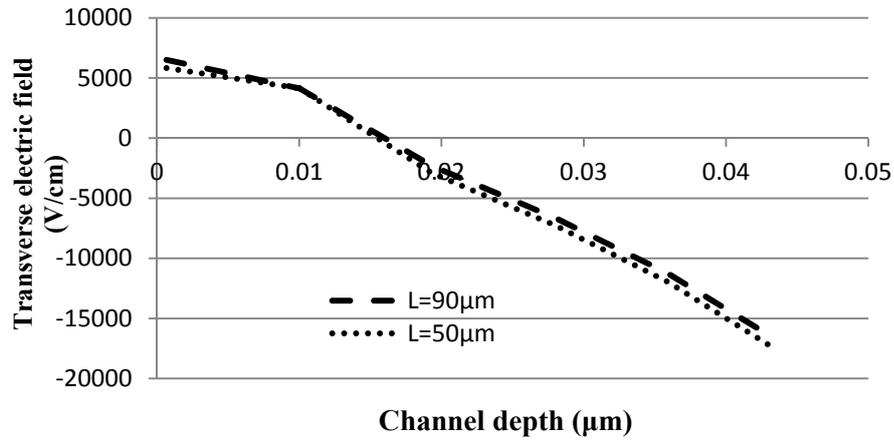
Figure 8: Channel length dependence on Transverse electric field
