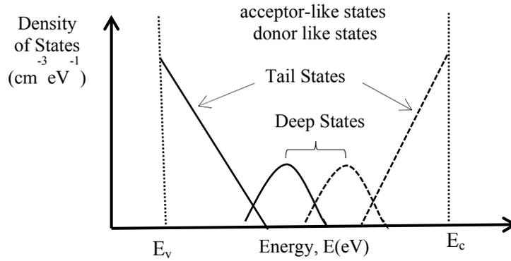
Figure 1: Density of states within the band gap of nc-Si
