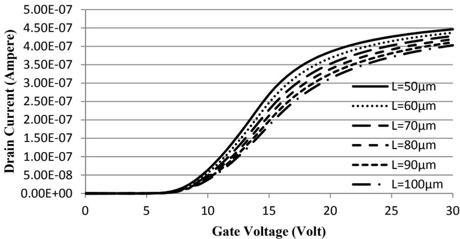
Figure 7: Variation of drain current as a function of gate voltage for different values of channel length
