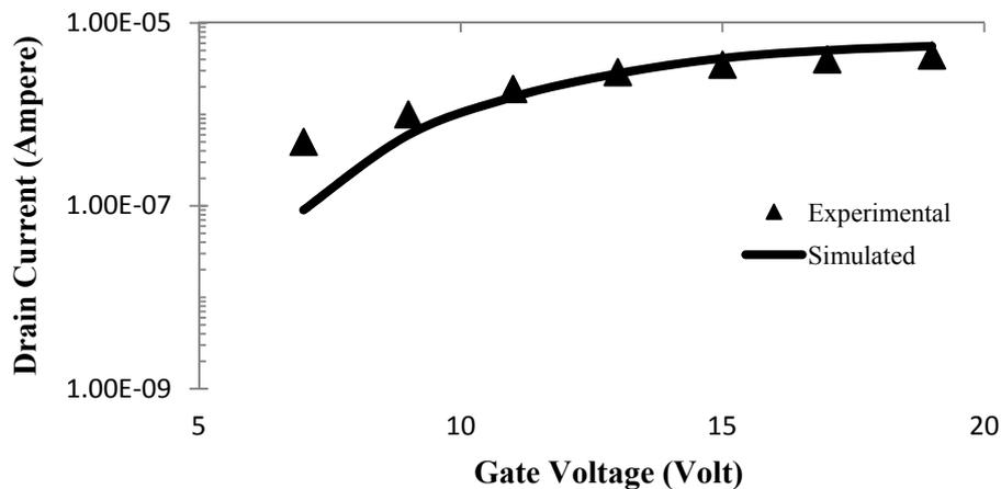
Figure 10: Plot of the transfer characteristic of nc-Si top-gated TFT ( $W=200\mu\text{m}$  and  $L=50\mu\text{m}$ ) simulated at  $V_{DS}=10\text{V}$  for  $WTA=0.02$  and  $R=10^6 \Omega$ . Solid line shows the experimental results of C.H.Lee et. al. [30] and dotted line shows simulated results
