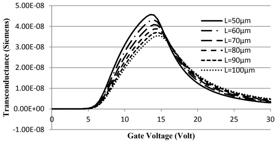
Figure 6: Variation of transconductance as a function of gate voltage for different values of channel length
