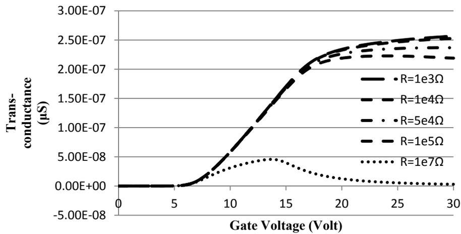
Figure 9: Variation of transconductance as a function of gate voltage for different values of parasitic resistance
