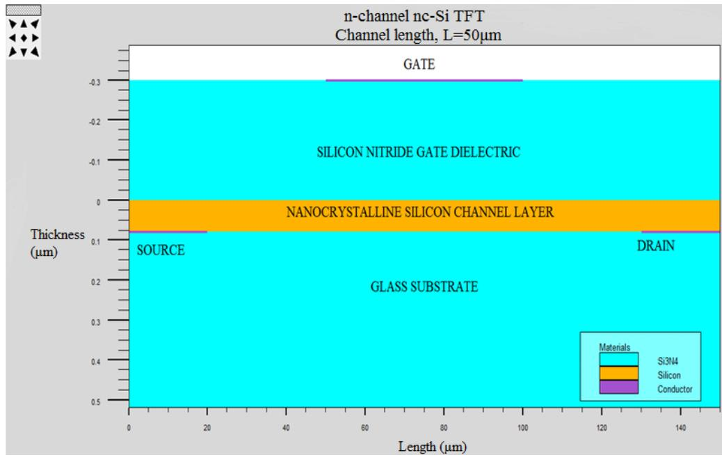
Figure 3: nc-Si TFT structure for ATLAS simulation
